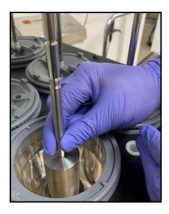
5.2.5 Install the Safety Clip to secure the upper and lower shafts.
