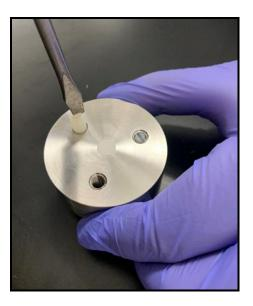
4.9 Screw the 8mm Intrinsic Die onto the Shaft and Holder assembly.
