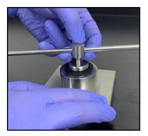
4.7 Remove the bolts from the bottom of the surface plate and carefully lift off the die and punch assembly. Remove any loose powder from the surface of the compact and die by using compressed air or nitrogen.
